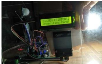
Figure 11. The RFID module detects unregistered cards.
